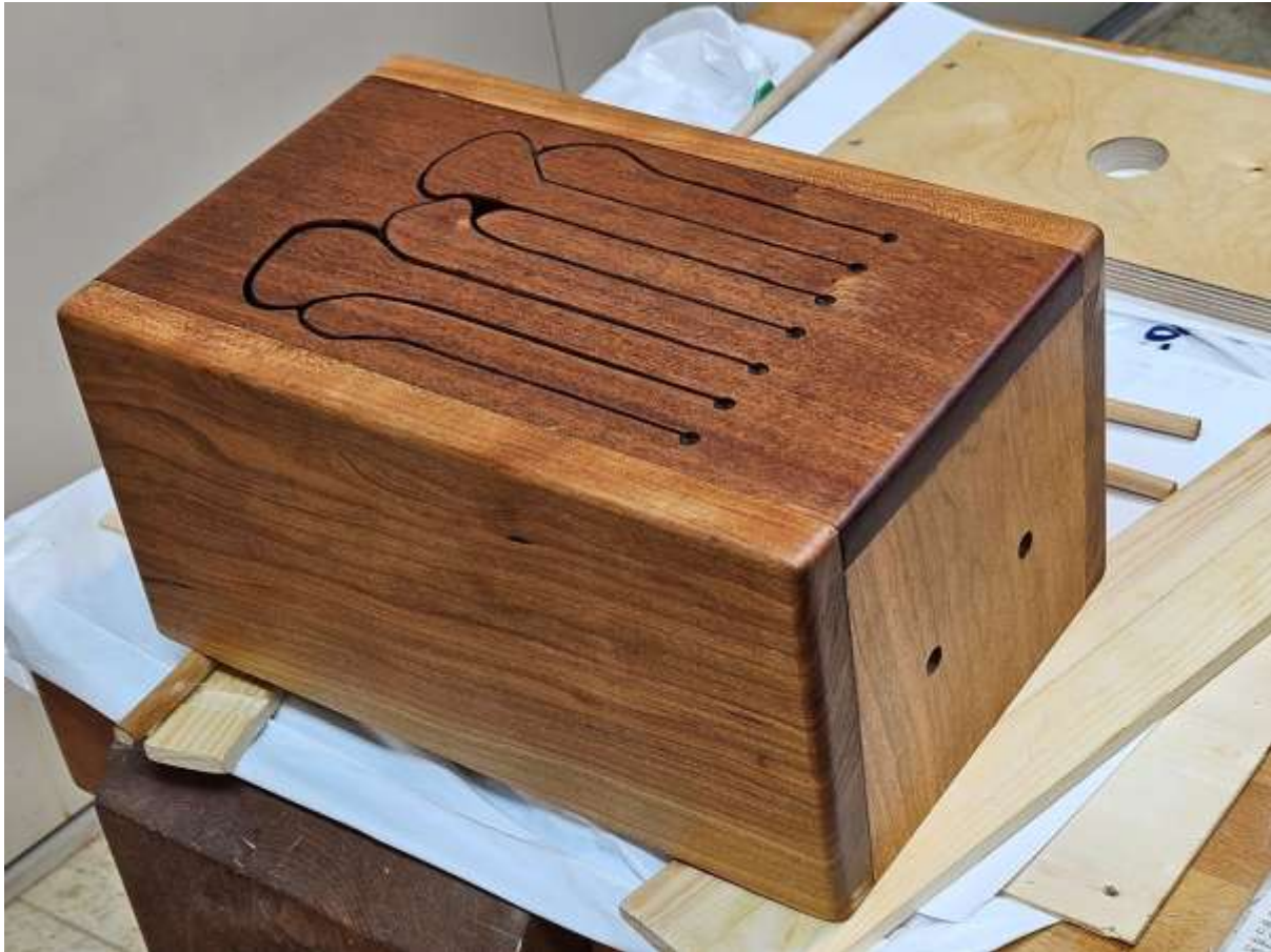
The drum waiting for the finishing oil to polymerize
